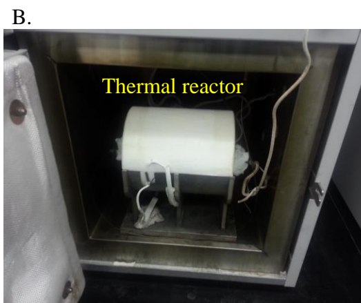
Figure 2.2 A. Varian CP-3800 gas chromatographic oven, B. thermal reactor inside the oven, and C. quartz reactor containing the catalyst.
