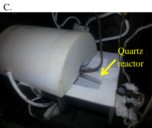
Figure 2.2 A. Varian CP-3800 gas chromatographic oven, B. thermal reactor inside the oven, and C. quartz reactor containing the catalyst.
